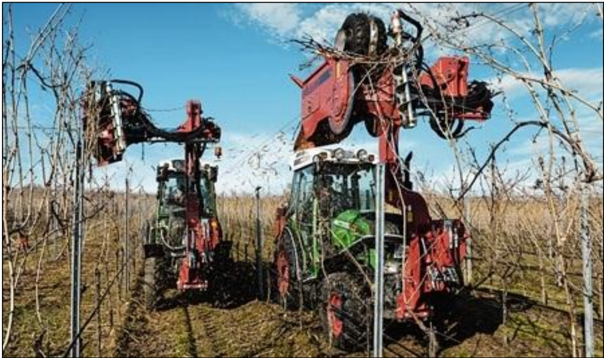
Figure 10: Front-mounted crop treatment machinery mounted on T2 vineyard tractors
