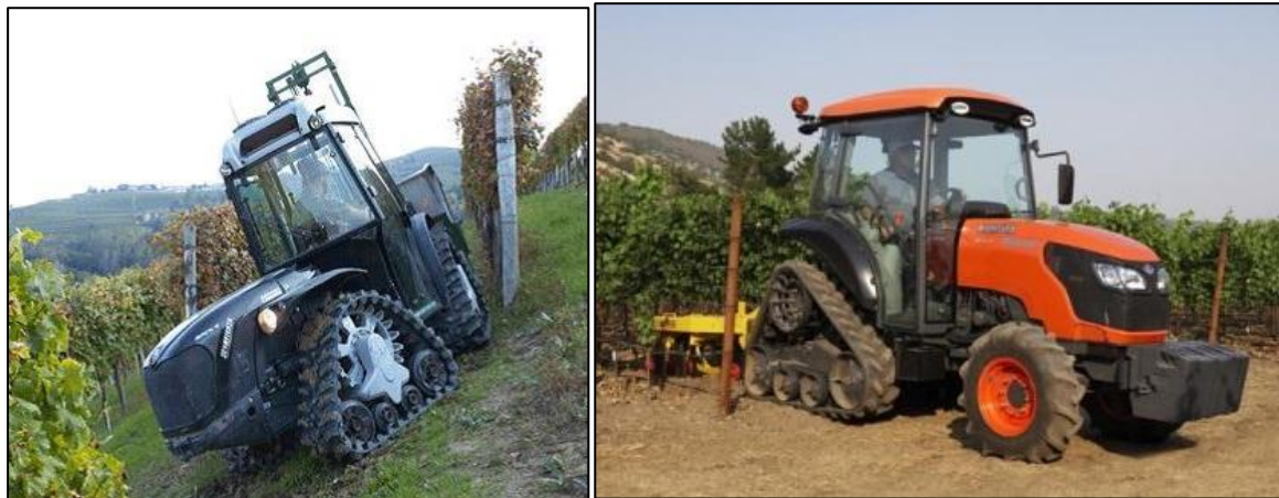
Figure 16: Full-track (left) and half-track (right) conversions of wheeled T2 tractors
