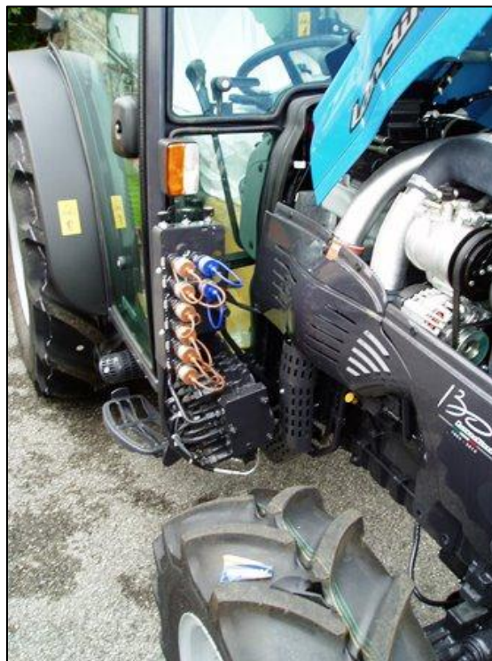
Figure 9: Mid-mounted external hydraulic couplings on a rigid-chassis T2 tractor
