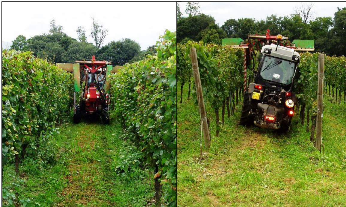
Figure 12: Front-mounted twin-row vine leaf trimmer hydraulically powered from tractor rear-mounted external couplings. Note adjustment of implement orientation relative to tractor chassis to compensate for sloping ground (lower right)
