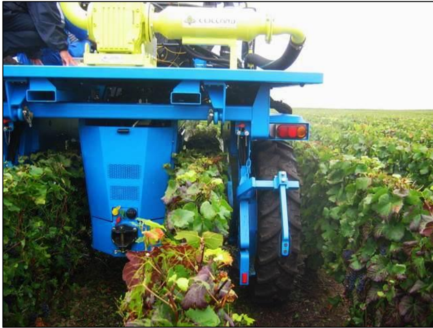
Figure 48: Degree of crop - machine clearance present as a T4.1 tractor undertakes leaf trimming operation in a vineyard
