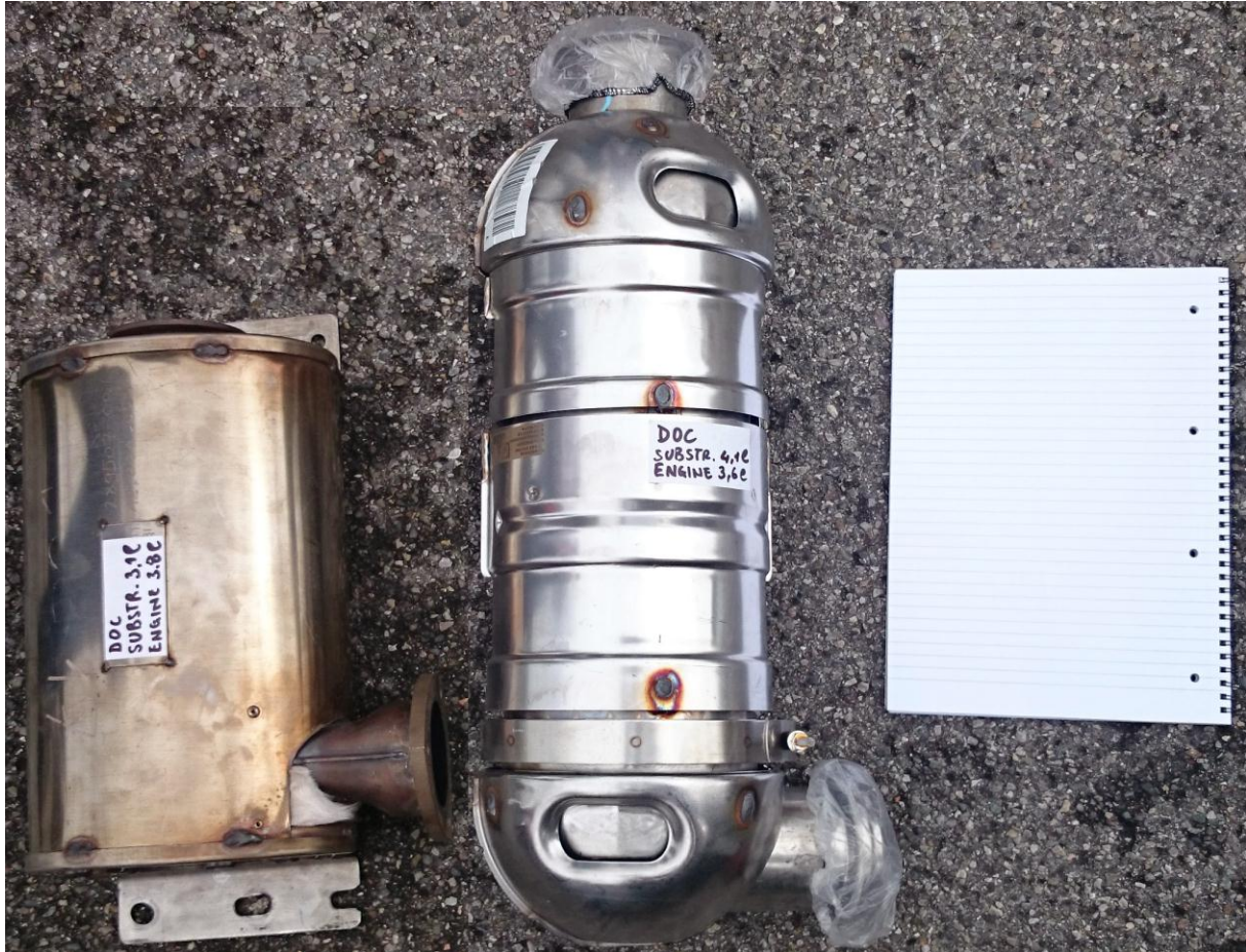
Figure 26: Tractor industry development to reduce DOC size (A4 paper for scale)
