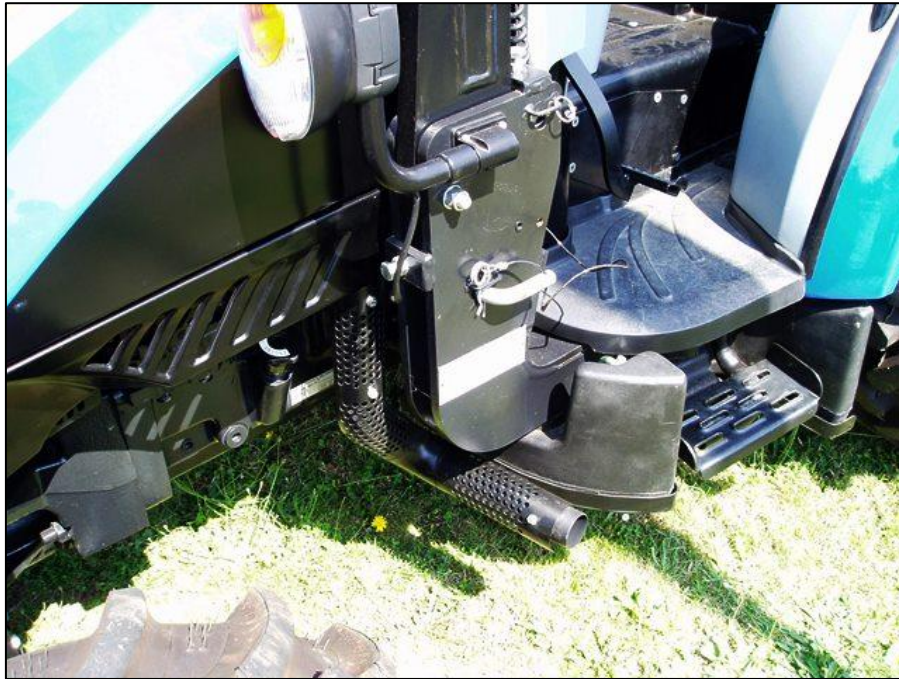
Figure 34: Stage IIIA T2 tractor plastic diesel tank moulded to fit around footstep and mid-mounted ROPS support brackets
