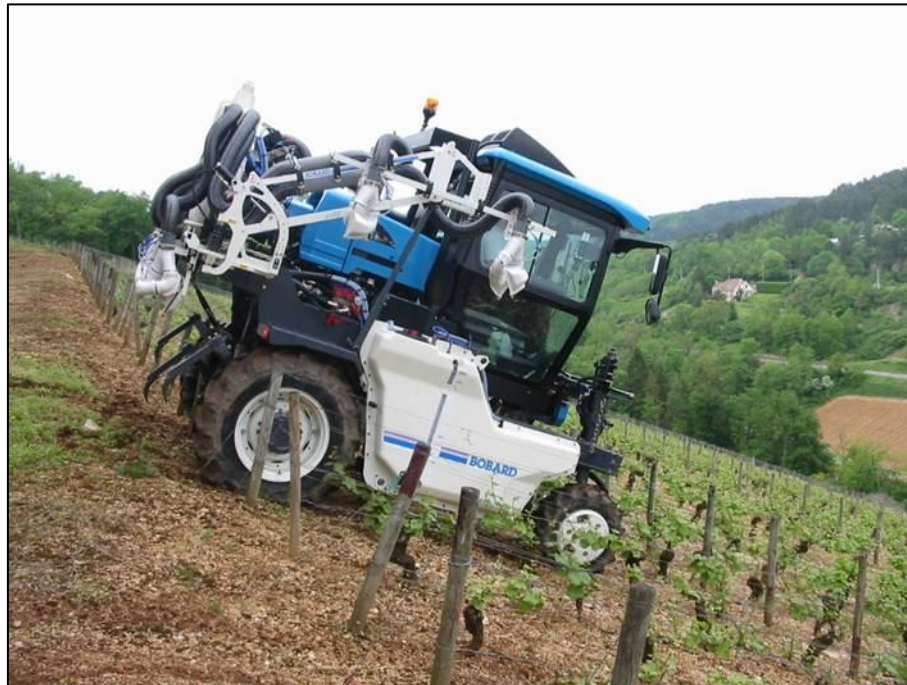
Figure 49: T4.1 tractor fitted with crop spraying equipment and saddle spray tanks
