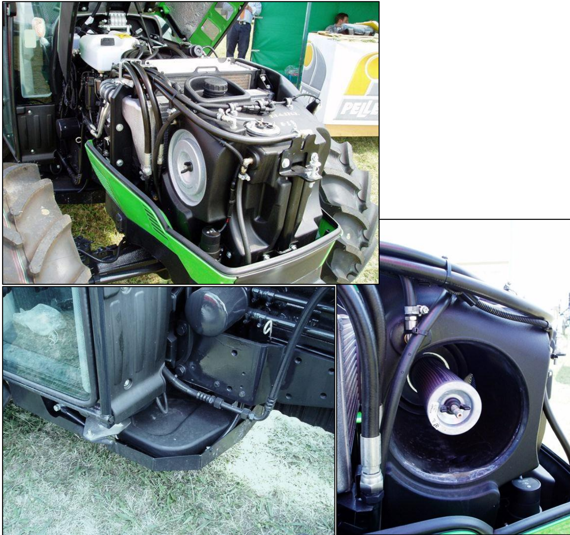
Figure 35: Front-mounted moulded plastic fuel tank on Deutz-Fahr T2 orchard tractor (top), incorporating integral engine air cleaner assembly (right). Reduced (55 litre) capacity supplemented by 40 litre belly-mounted fuel tank (bottom left)
