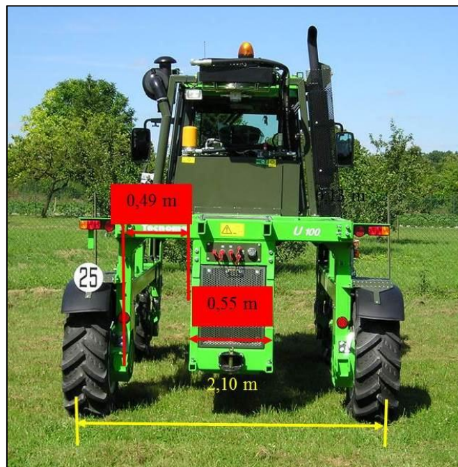
Figure 47: Typical dimensions of a T4.1 tractor with low, centrally-mounted engine, configured to work in 1.05 m wide rows
