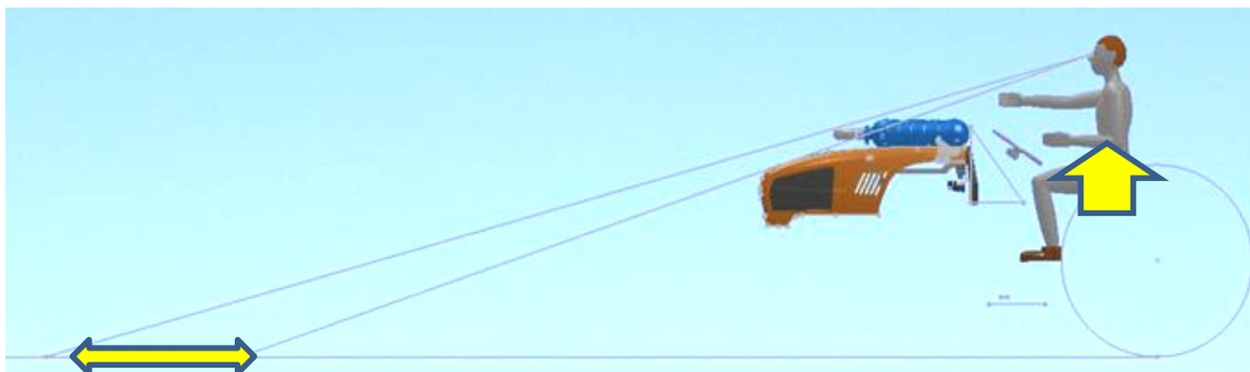
Figure 42: Over bonnet visibility with additional EAT hardware. Loss of viewing area negated with seating position change
