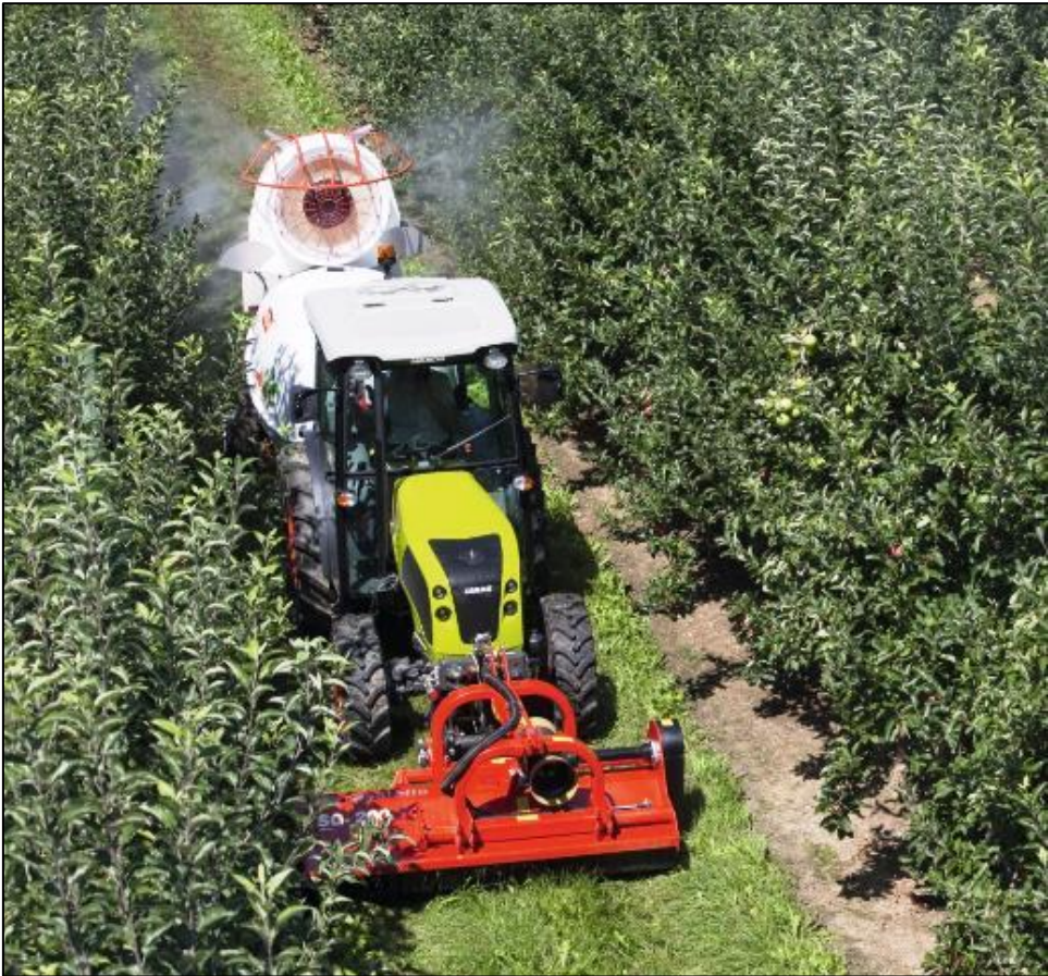
Figure 13: Air-assisted sprayer applying agrochemicals and mowing in an orchard
