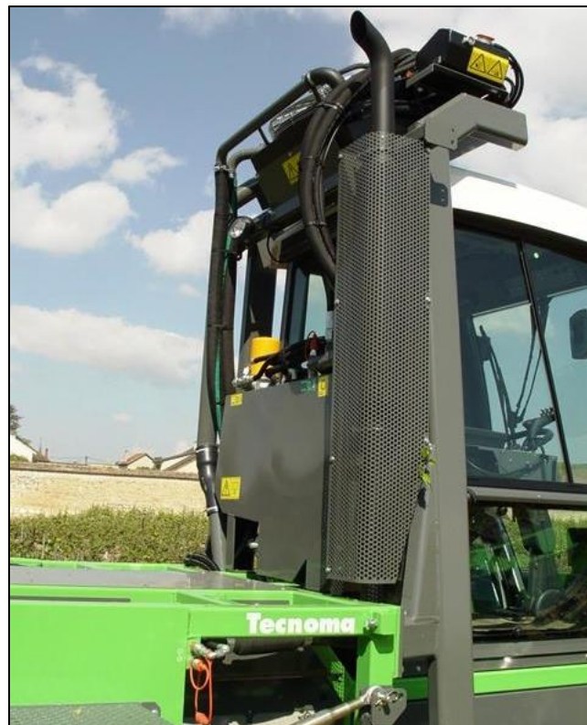
Figure 50: Area behind cab and exhaust system on a Stage IIIA T4.1 high-clearance tractor
