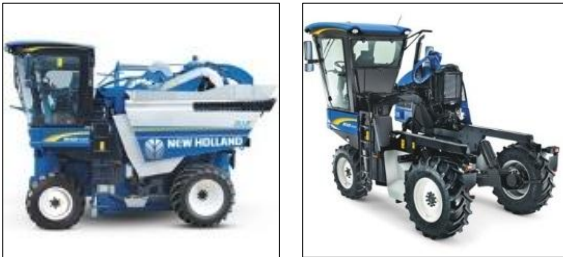
Figure 23: Self-propelled grape harvester with demountable harvesting equipment. Harvesting unit fitted (left) and removed (right) to accept other equipment
