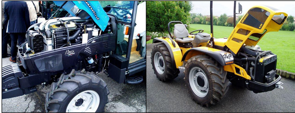
Figure 43: Stage IIIA T2 tractor front-of-engine detail - 81 kW rigid-chassis (left) and 68 kW articulated chassis (right)
