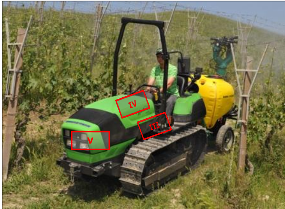
Figure 45: Some possible locations for EAT hardware on C2 track-laying tractors
