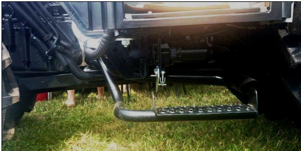
Figure 39: Area under the cab floor on a conventional, rigid-chassis T2 tractor
