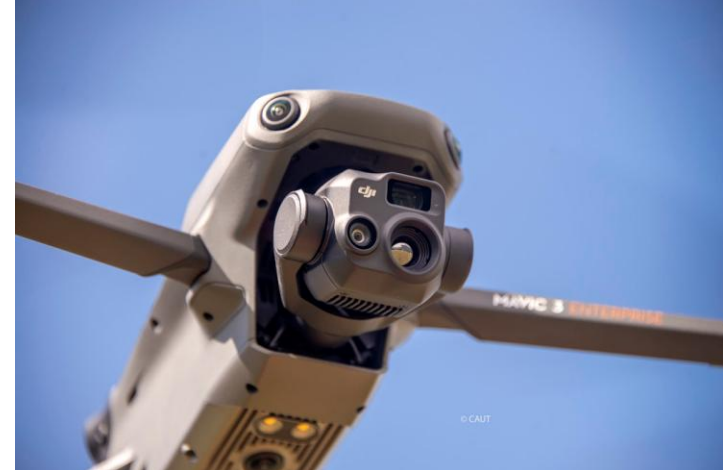
Mavic 3 T (M3T) – DJI Camera Termica + RGB 20MP
