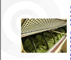
In addition, this operation disrupts a proportion of the oily cells remained unbroken during the crushing, allowing the recovery of another oil fraction.
