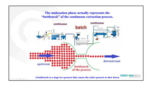
Currently the system used to guarantee continuity to the process, without interrupting the activity of the machines upstream and downstream of the malaxer, consists in placing several malaxing machines in parallel, with an heavy economic investment.
